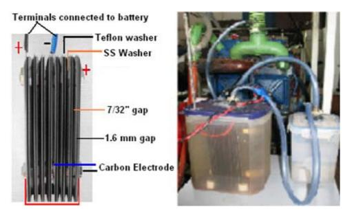
Figure 1. Arrangements of electrodes in first design of electrolyser.
