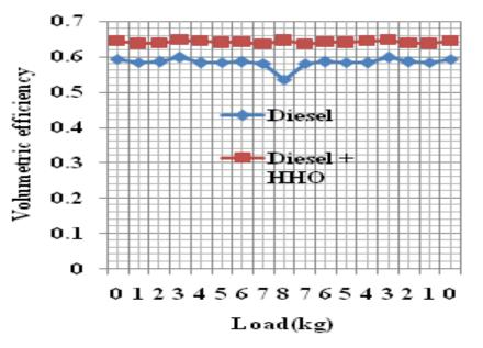
Figure 8. Graph of volumetric efficiency in percent v/s load in kg.
