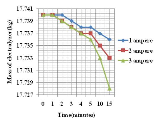
Figure 5. Graph of mass of electrolyser v/s time.
