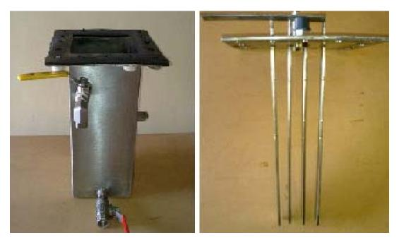
Figure2. Arrangements of electrodes in second design of electrolyser.
