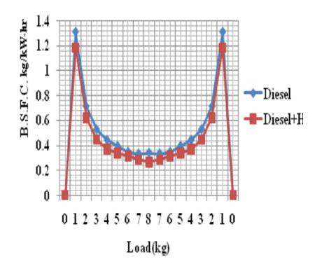
Figure 6. Graph of brake specific fuel consumption in kg/kW-h v/s load in kg.
